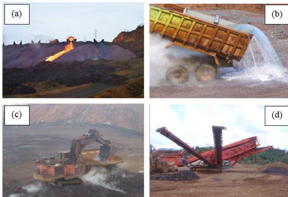
Figure 2. Processing of air-cooled ferronickel slag (ACFS) aggregate: (a) dumping; (b) cooling; (c) gathering; and (d) crushing.
